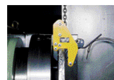
TWG modified side plates for use in confined spaces (e.g. lathe machine).
